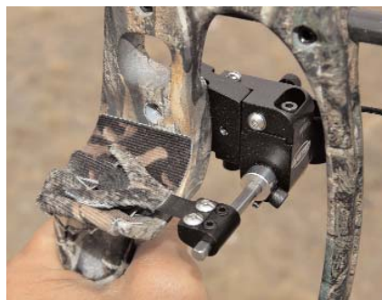
One key feature to Arizona Archery's Avalanche rest is its Whale Tail launcher. It's made of flexible steel, which dampens arrow oscillation at take off, providing a smoother, more forgiving shot and easier paper tuning.
